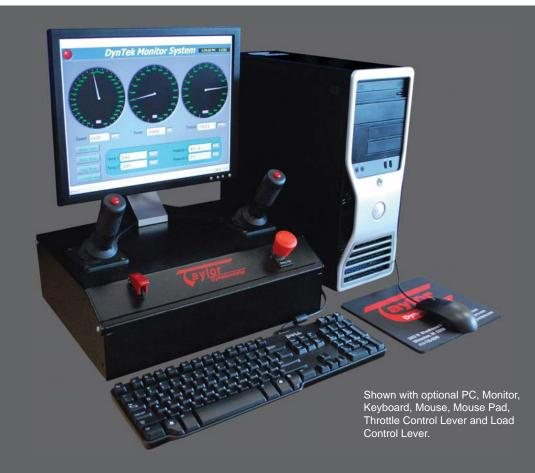
The DynTek-PC engine dynamometer instrumentation system is a display only system intended for basic engine dynamometer testing requirements. This system provides for the measurement of torque in either tension or compression (both clockwise and counter-clockwise engine rotation) and speed from a standard Magnetic Pickup. The system is designed to set on a table or desktop near the PC.
