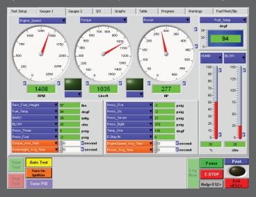
DynPro provides the flexibility and control required in today's challenging test environment, gives the operator complete control of the dynamometer functions and provides comprehensive data acquisition. DynPro controls and acquires the data from the many accessories that compliment Taylor's DynPro system, including the Smoke Opacity Meter, the **Emissions Gas** Analyzer, the Pressure and Temperature Package, the Heavy-Duty Electronic Interface
